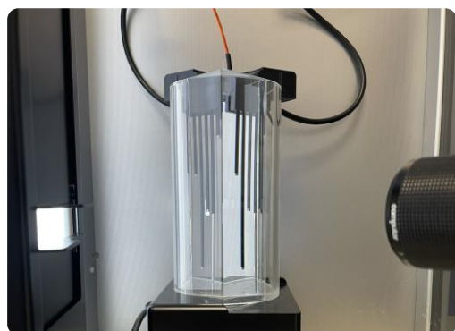
Fig1. FOAMSCAN™ configuration for foams generated externally and sampled by pouring
