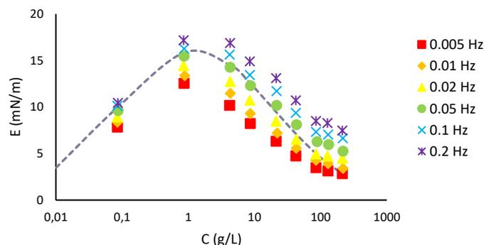
Viscoelastic modulus  $E$  as functions of concentration of AOSB537 bitumen-in-toluene/NaHCO<sub>3</sub> with increasing frequency. Data from [2]. The dotted curve represents the schematic evolution of  $E$  as a function of  $C$  [3]
