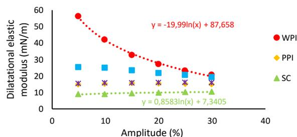
Apparent dilatational elastic moduli at the air-water interfaces stabilized by proteins and protein blends as a function the applied deformation (frequency, 0.01 Hz). Data from [4]
